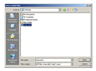
**NOTE (4 button box only):** You can add up to 4 different sound files. The sounds will play in the order that they are listed. The first sound listed is activated by the first button ("key 1") attached to the box. The second sound listed, the second button—and so on. You can use the **MOVE UP**, **MOVE DN** and **DEL FILE** buttons to edit the playlist.
