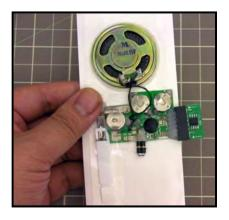
Remember to hold the chip by the sides. Try not to touch the chip surface.
