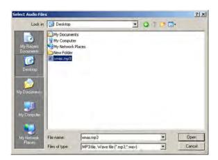
**NOTE:** You can load as many sound files up to the number of buttons/switches your module has. For example, if your module has 3 buttons, you can load 3 sound files. Each sound file loaded will play on a different button. You can use the **MOVE UP**, **MOVE DN** and **DEL FILE** buttons to edit the playlist and arrange which sound plays on which button.
